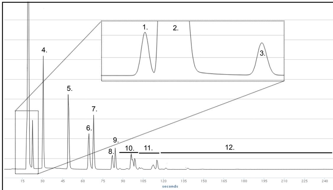
Column: Rt-Q-Bond, 8 m, Variable Volume Injector
