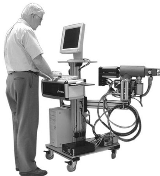
Figure 1: Example of a Mobile Sampling System
