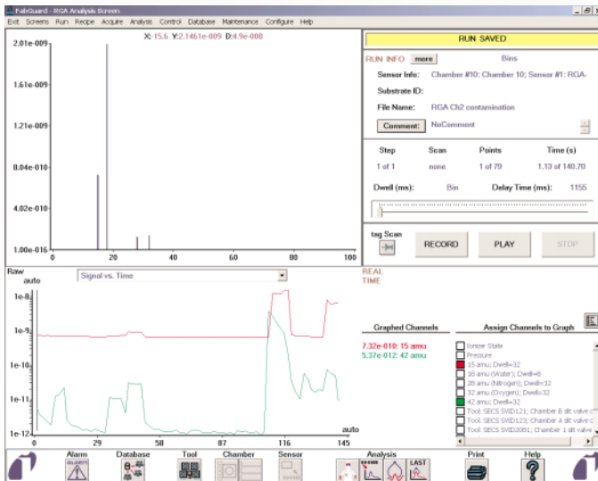
Figure 1. RGA data for several wafers moving through the Transfer Chamber. Masses 15 and 42 are plotted.
