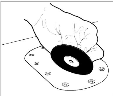
1.4 Press firmly around the entire tape ring. Work around the ring several times.
