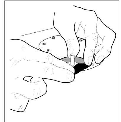
4.1 To minimize risk of damage to paint start peeling at the outer edge.
