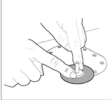
1.5 Leave the pad to set for at least 10 minutes before purging and injecting gas.
