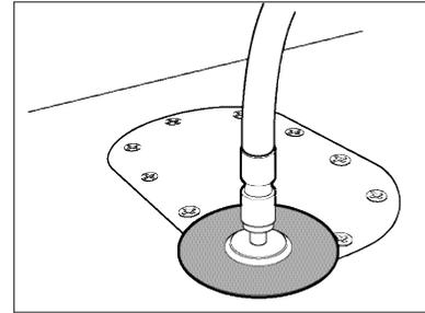
3.7 Increase output pressure slowly to desired pressure (max 0.5 bar / 7.2 psi).
