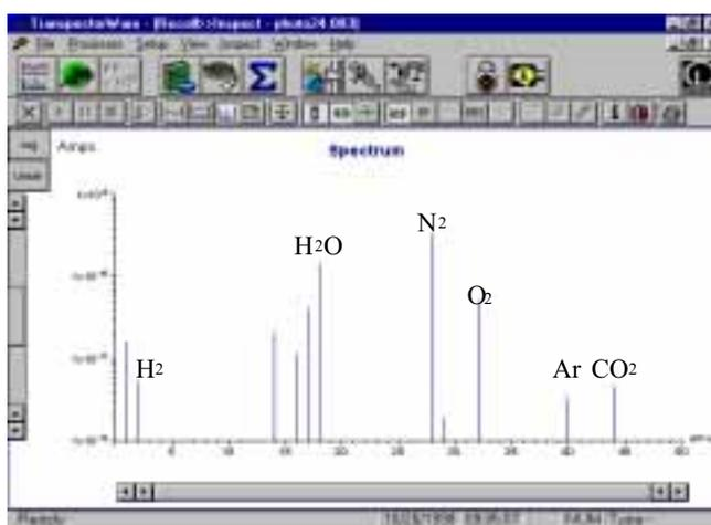
**Figure 1: Air and Water Contamination Spectra**
