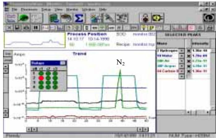
**Figure 4: An Air Excursion (Mass 28) Activates the Upper Setpoint Of Relay #1**
