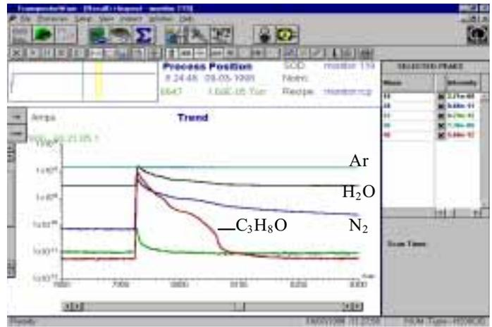
**Figure 3: Isopropyl Alcohol and Air Contaminating a Process**
