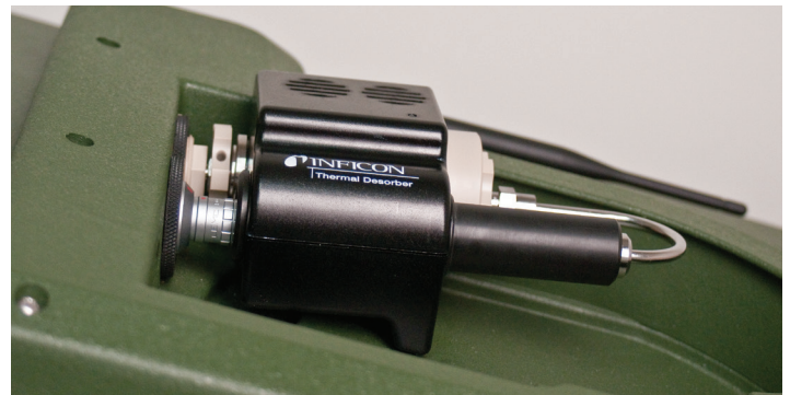
Thermal Desorber connected to the HAPSITE ER universal interface
