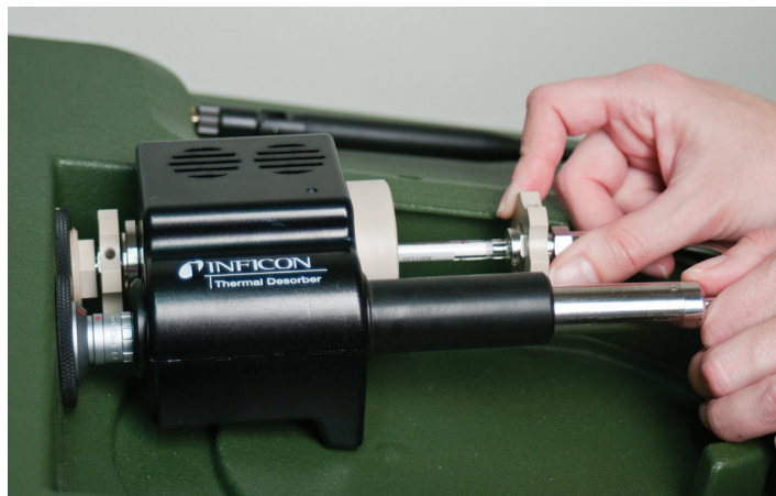
Simply load the tube into the Thermal Desorber for quick analysis
