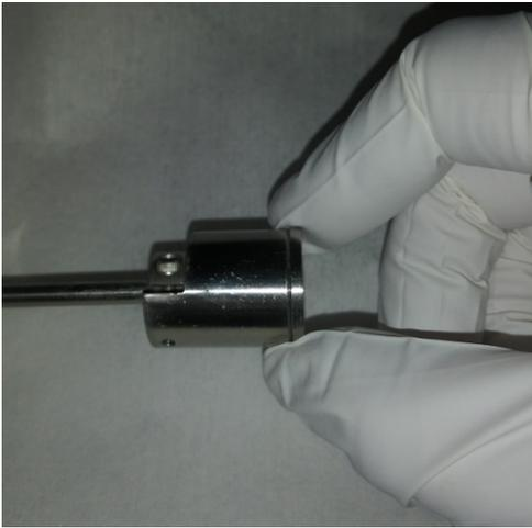
9. Install the QCM sensor back on the foreline with a KF40 clamp and the appropriate centering ring.
