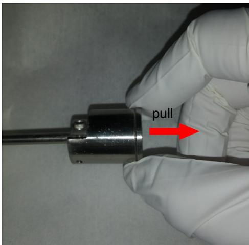
3. Insert the tapered end of a crystal snatcher (PN 008-007) into the ceramic retainer as shown below and apply a small amount of pressure. This locks the ceramic retainer to the snatcher and allows the ceramic retainer to be pulled straight out.
