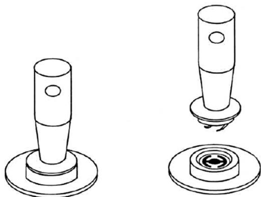
4. Invert the crystal holder to allow the crystal to drop out.
