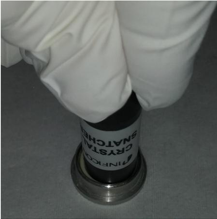
8. Reinstall the crystal holder into the sensor body by pressing the crystal holder straight in, making certain that the crystal holder is completely seated in the sensor body. Some force may be required.
