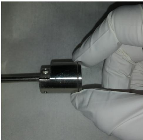
4. Install the QCM sensor back on the foreline with a KF40 clamp and the appropriate centering ring.
