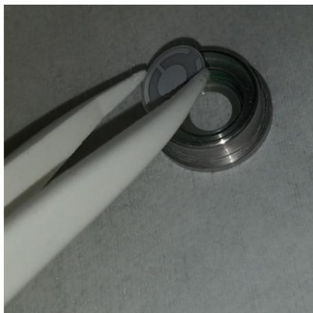
6. Replace the ceramic retainer. Initially orient the ceramic retainer at an angle to display the spring wire segments in the crystal holder. Avoid using excessive force when handling the ceramic retainer to prevent breakage. Avoid rotating the ceramic retainer after installation, to prevent scratching the crystal electrode.
