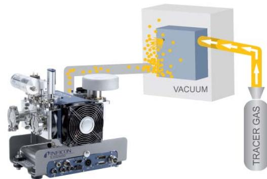
*Battery cells prefilled with helium are typically tested via vacuum chamber leak detection. This process is very common for prismatic battery cells.*
