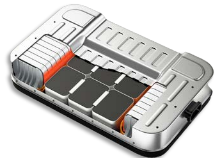
Battery packs in electrical vehicles need to be tested for loss of cooling fluid and against intake of water.
