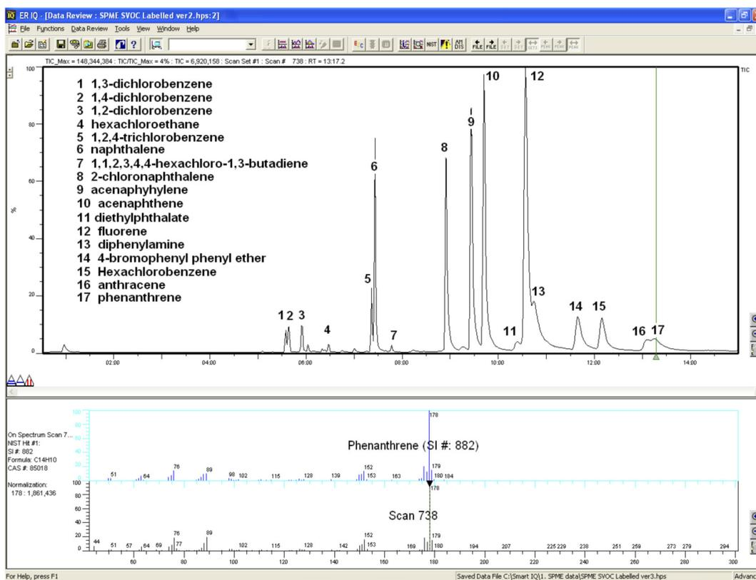
Column: Rtx-1MS (15 m x .25 mm x 1.0 µm)
