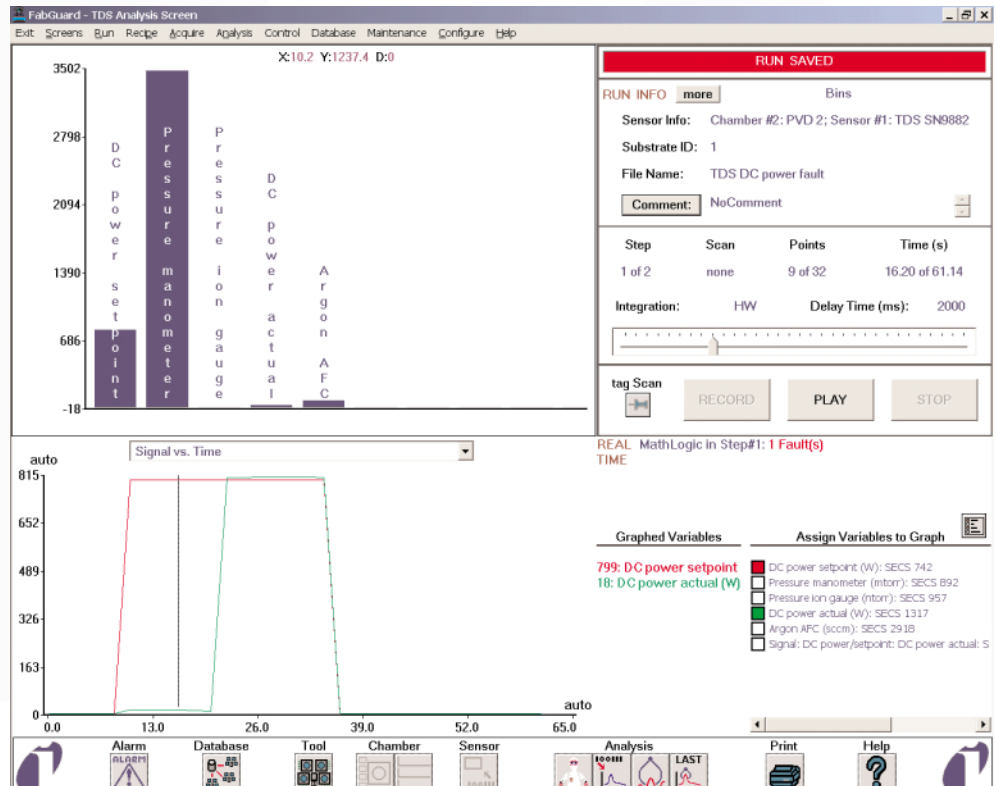
Figure 1 - Data collected by a Tool Data Sensor for one wafer during a PVD process.
