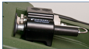
Thermal Desorber connected to the HAPSITE ER universal interface
