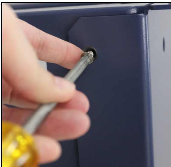
Figure 7 Use screws to attach unit to brackets
