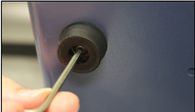
Figure 1 Remove rubber feet from Micro GC Fusion
