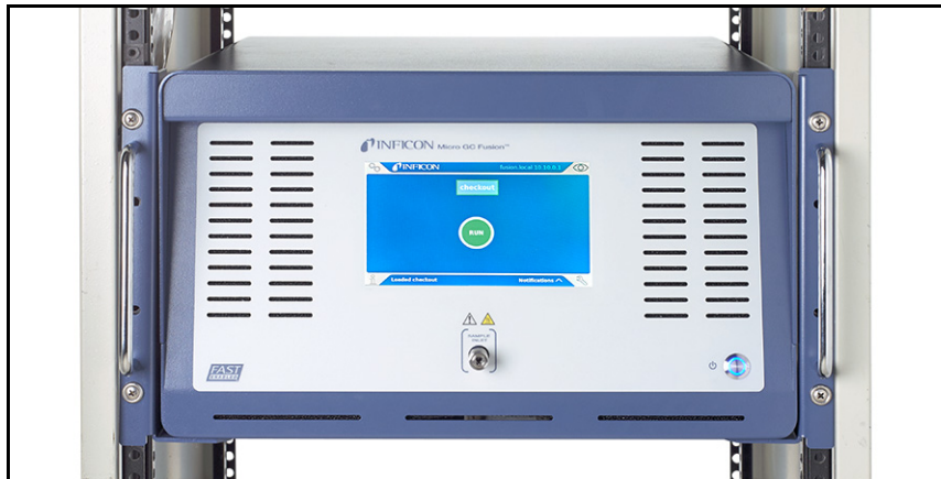
Figure 5 Micro GC Fusion set on mounting brackets
