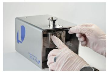
13. Using the 5/16 in. wrench, reconnect the RF cable to the MSC. Be sure not to overtighten the cable or damage could occur to the MSC.
