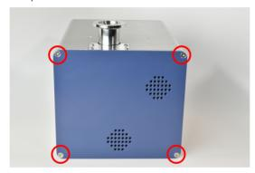
3. Using a 2 mm hex driver, remove the flange plate by removing the four screws. Keep the flange plate and screws for reassembly at the end of this procedure.
