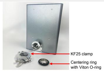
2. Using a 2 mm hex driver, remove the front end plate by removing the four screws. Keep the front end plate and screws for reassembly at the end of this procedure.
