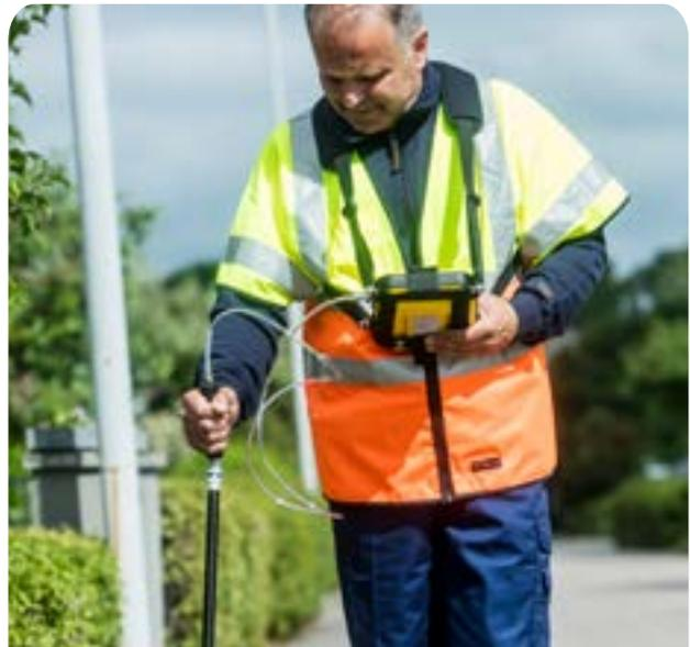
IRwin is a portable methane leak detector with in-built gas chromatograph (GC) for easy and fast ethane analysis.
