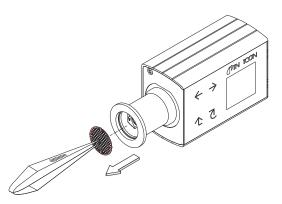
2 Carefully place the baffle onto the sensor opening.
