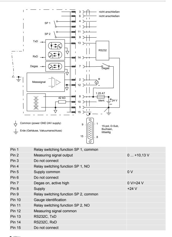
For cable lengths up to 5 m (0,34 mm<sup>2</sup> conductor cross-section) the output signal can be measured directly between the positive signal output (Pin 2) and supply common GND (Pin 5). At greater cable lengths, differential measurement between signal output (Pin 2) and signal common (Pin 12) is recommended.
