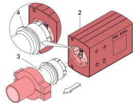
**4** Slide the electronics unit in to the mechanical stop and lock it with the hexagon socket set screw.
