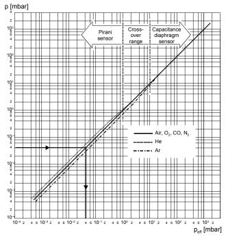
Calibration in pressure range  $2 \times 10^{-2} \dots 1$  mbar
