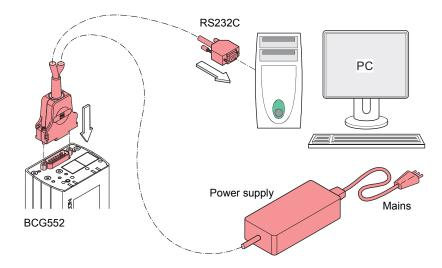
3 Connect the power supply to the mains.
