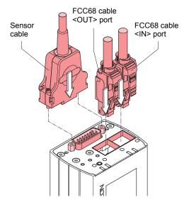
2 Secure the sensor cable connector using the lock screws.
