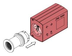
Installing the electronics unit
