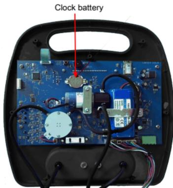
To replace the cell, carry out the following procedure.
