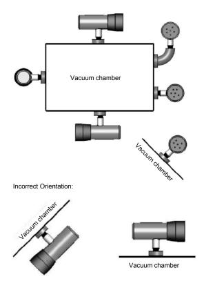
Mount the PGE050 with port down, if possible, to help minimize the effect of any particles or condensation from collecting in the gauge.
