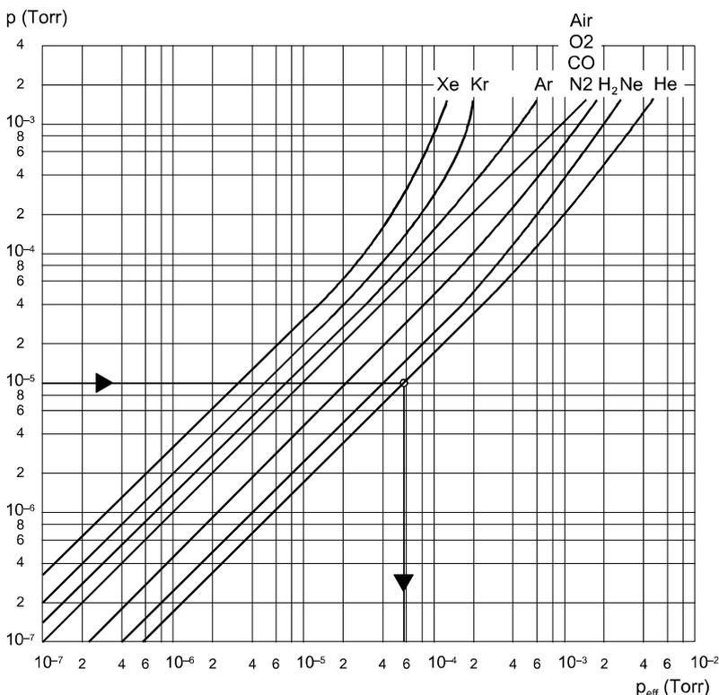
In the range below 10<sup>-5</sup> Torr the pressure indication is linear. For gases other than air / N<sub>2</sub>, the pressure can be determined by means of the following conversion formula:
