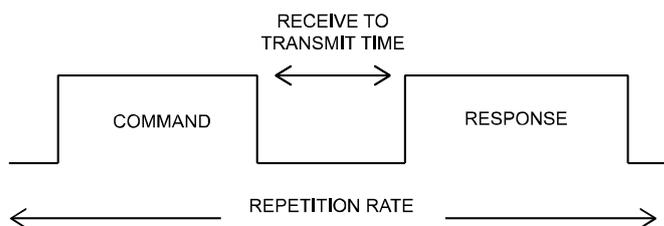
The maximum command repetition rate will depend on the length of the command sent and the response received, as well as the baud rate. The maximum repetition rate for the baud rate you are using can be found in the following table:
