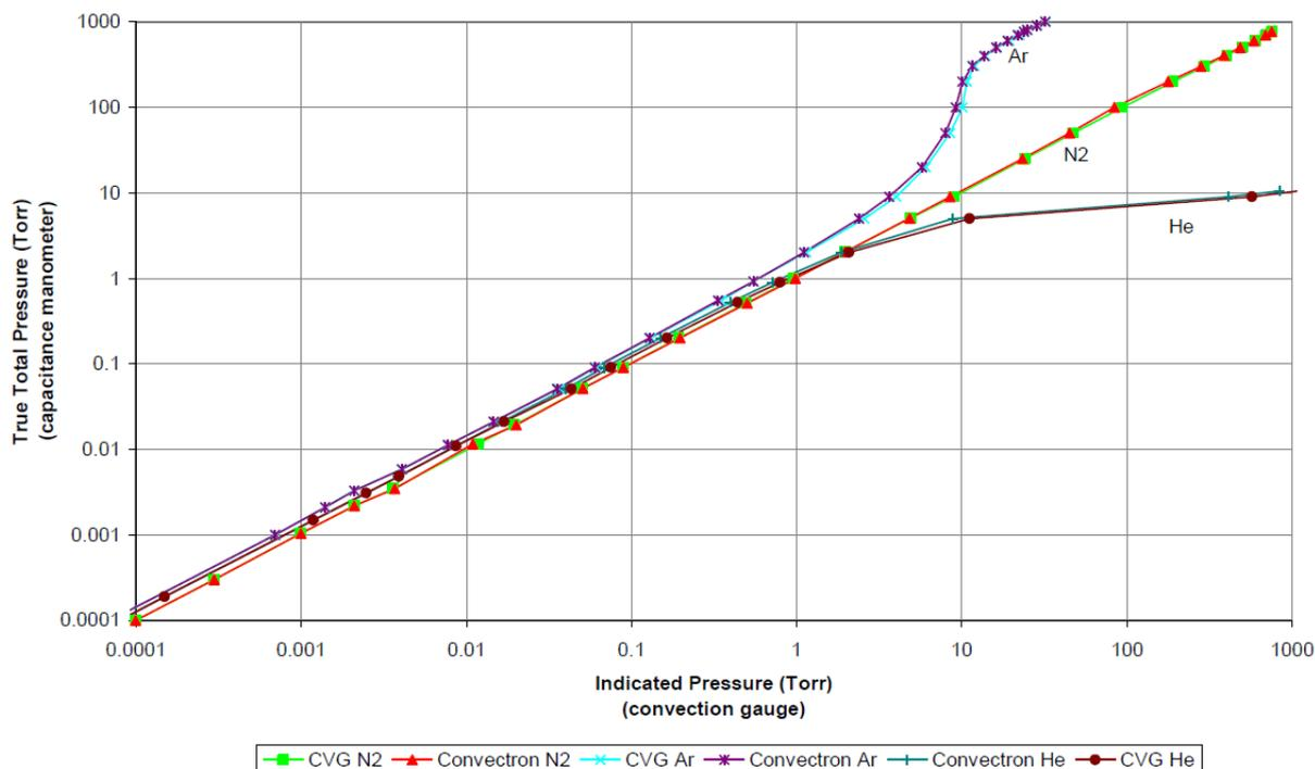
The Y-axis of the above chart is actual pressure as measured by a capacitance manometer, a diaphragm gauge that measures true total pressure independent of gas composition. The X-axis is the pressure reading indicated by the convection gauge under test. This chart shows readings for an INFICON convection gauge (CVG) and Granville-Phillips® Convectron® gauge to illustrate that the difference in the response for both of these types of gauges is virtually indistinguishable.
