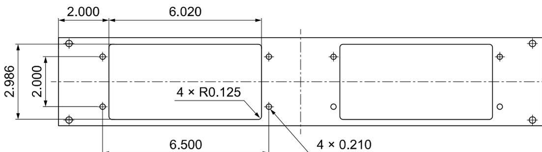
The single cut-out and dual cut-out rack mountable panels shown above are available from INFICON. Panel color matches the front panel of VGC083C units. Screws for mounting to rack enclosure are included.
