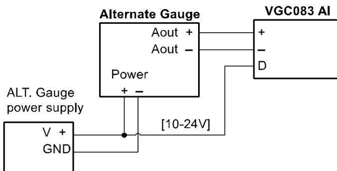
An Auxiliary Power Supply is required for your Alternate Gauge, e.g., a CDG. Ensure power is applied to your Alternate Gauge before turning on the power to VGC083.
