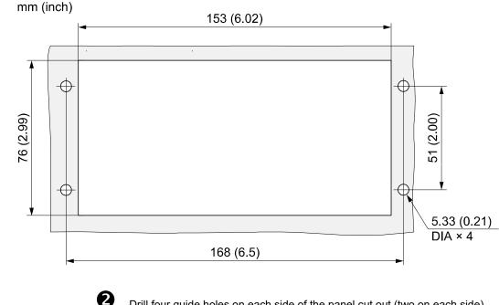
Drill four guide holes on each side of the panel cut out (two on each side) with dimensions as shown in the panel cut-out drawing above.
