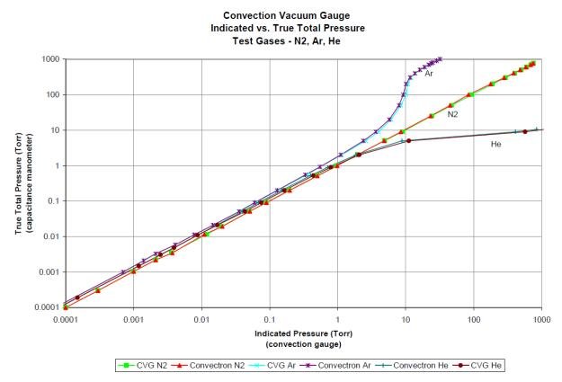
The Y- axis of the above chart is actual pressure as measured by a capacitance manometer, a diaphragm gauge that measures true total pressure independent of gas composition. The X-axis is the pressure reading indicated by the convection gauge under test. This chart shows readings for an INFICON convection gauge (CVG) and Granville-Phillips<sup>®</sup> Convectron<sup>®</sup> gauge to illustrate that the difference in the response for both of these types of gauges is virtually indistinguishable.
