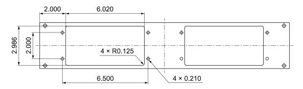
The single cut-out and dual cut-out rack mountable panels shown above are available from INFICON. Panel color matches the front panel of VGC083C units. Screws for mounting to rack enclosure are included.
