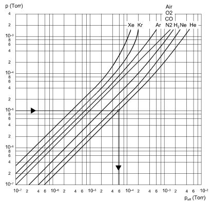
In the range below  $10^{-5}$  Torr the pressure indication is linear. For gases other than air / N2, the pressure can be determined by means of the following conversion formula:
