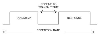
The maximum command repetition rate will depend on the length of the command sent and the response received, as well as the baud rate. The maximum repetition rate for the baud rate you are using can be found in the following table:
