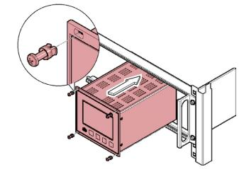
... and fasten the adapter panel to the rack chassis adapter using the screws supplied with the VGC094.
