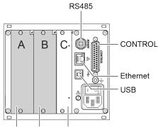
Measurement Interface and relay board boards
