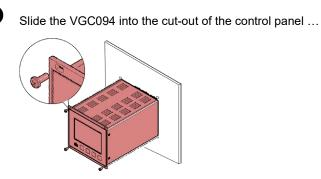
... and secure it with four M3 or equivalent screws.
