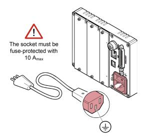
If the unit is installed in a switching cabinet, the mains voltage should be supplied and turned on via a central distributor.
