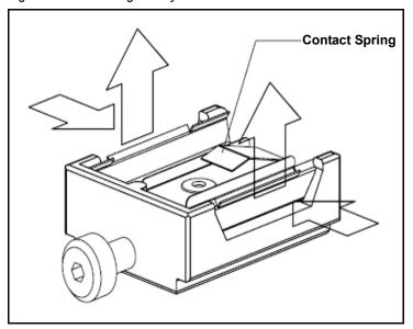
Figure 4-4 Replacing the crystal
