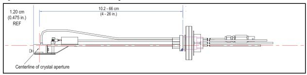
Figure 1-8 Right Angle Cool Drawer sensor length with shutter
