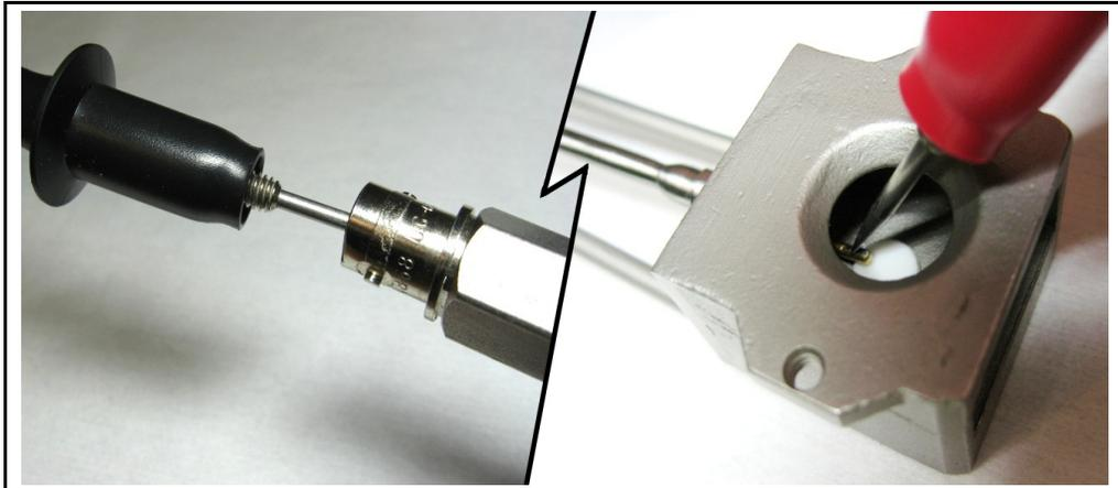
A very useful tool for rapidly evaluating the cause of a persistent "Crystal Fail" is the test crystal, which is included with each non-modelock oscillator package, this tool utilizes a packaged crystal at 5.5 MHz and a connector that allows the direct connection to BNC cables.
