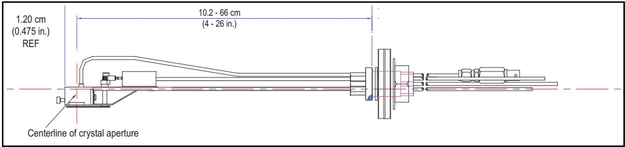
Figure 1-8 Right Angle Cool Drawer sensor length with shutter
