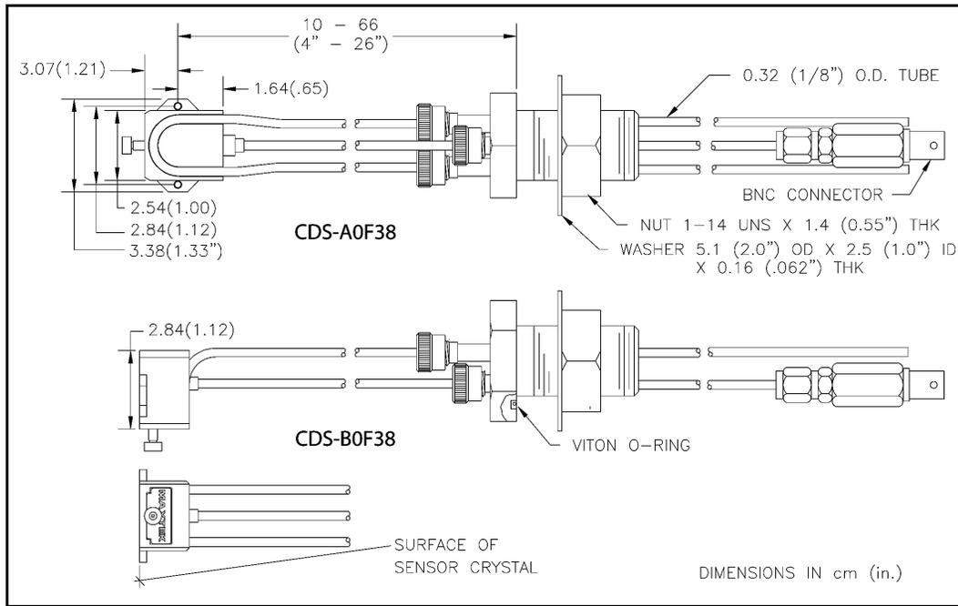
Figure 1-6 Cool Drawer sensors welded to CF 40
