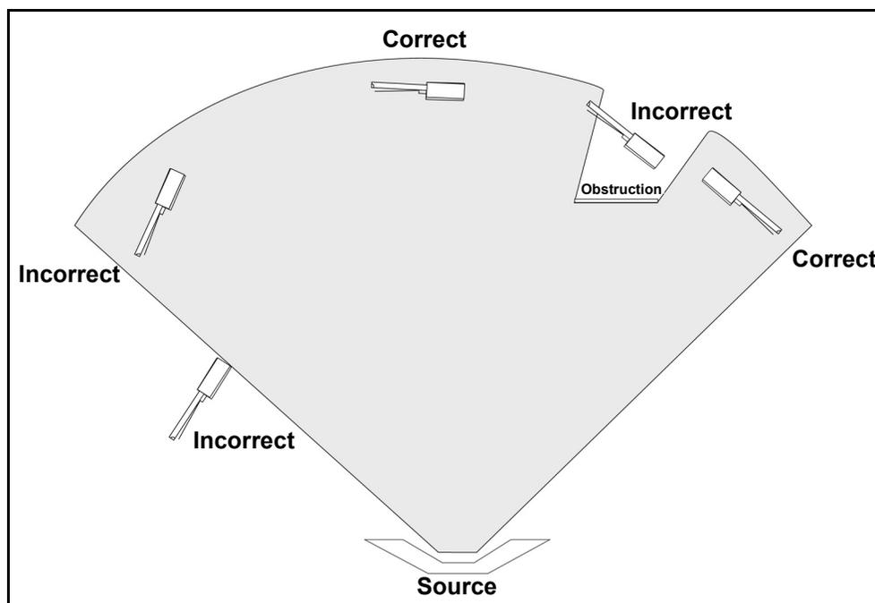
To guard against spattering, use a source shutter to shield the sensor during initial soak periods. If the crystal is hit with only a very small particle of molten material, it may be damaged and stop oscillating. Even in cases when it does not completely stop oscillating, the crystal may immediately become unstable, or shortly after deposition begins, instability may occur.
