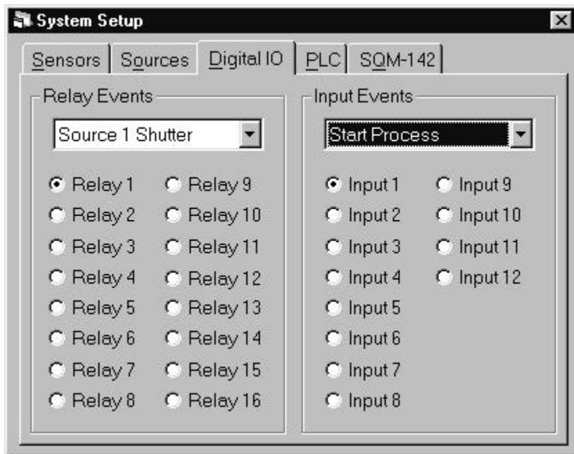
The SID-142 uses an inexpensive PLC to provide digital I/O capabilities. The Digital I/O tab assigns deposition events (i.e. open shutter, start deposit, final thickness, etc.) to the available relays and inputs on the PLC.
