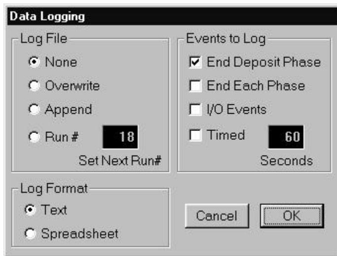
A number of “events” can trigger a data entry in the log file. “End Deposit Phase” records process data (rate, thickness, time, etc.) at the end of each layer’s deposit phase. Similarly, “End Each Phase” logs data at the end of each phase (conditioning, depositing, etc.). “I/O Events” logs data each time an external digital input or output changes. Finally, “Timed Logging” records data at the selected time intervals throughout the process.
