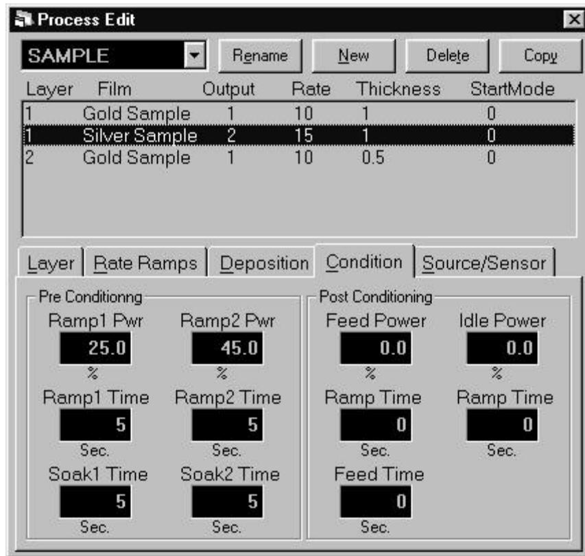
**Ramp 1:** Ramp power sets the power level desired at the end of the ramp phase, in % of full scale. Ramp time sets the time to ramp with a linear rate from the initial power to the Ramp power. Soak time sets the time the output remains at the ramp power level.
