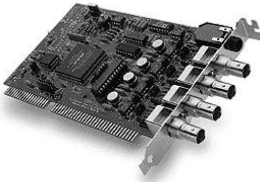
Sigma's SQM-142 card installs in a computer ISA slot, and provides the interface to the vacuum deposition system. Each card measures up to four quartz sensors via BNC inputs, and supplies the control signal for two evaporation sources via a dual phone plug output. Up to two cards can be installed in a computer, creating an eight input, four output, codeposition controller.
