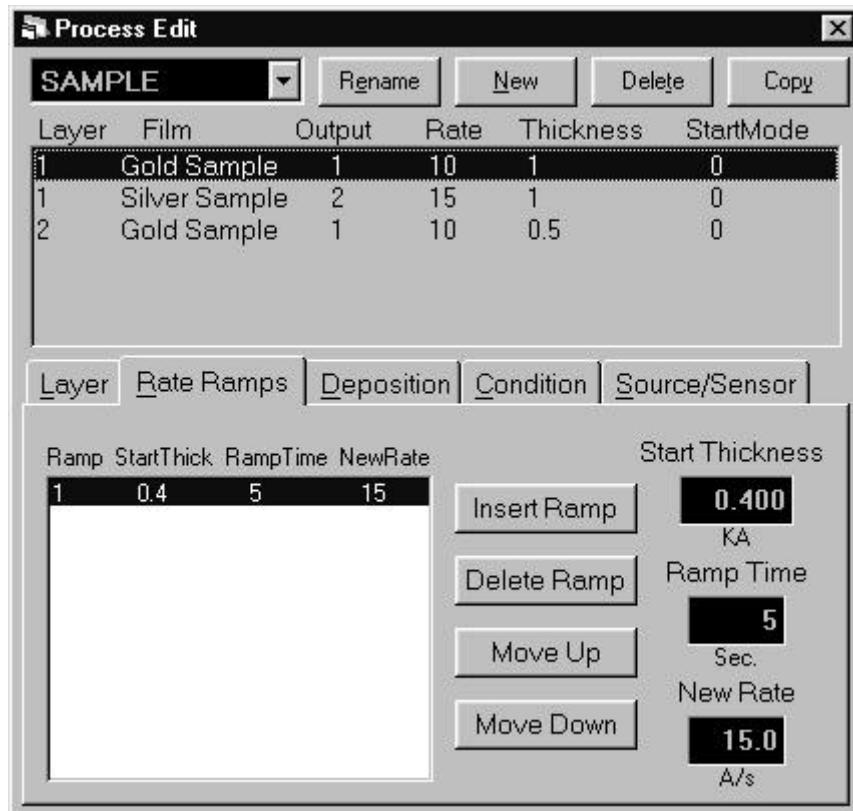
**Insert Ramp:** Inserts a new rate ramp for the selected layer, at the selected position. Existing rate ramps are shifted down.
