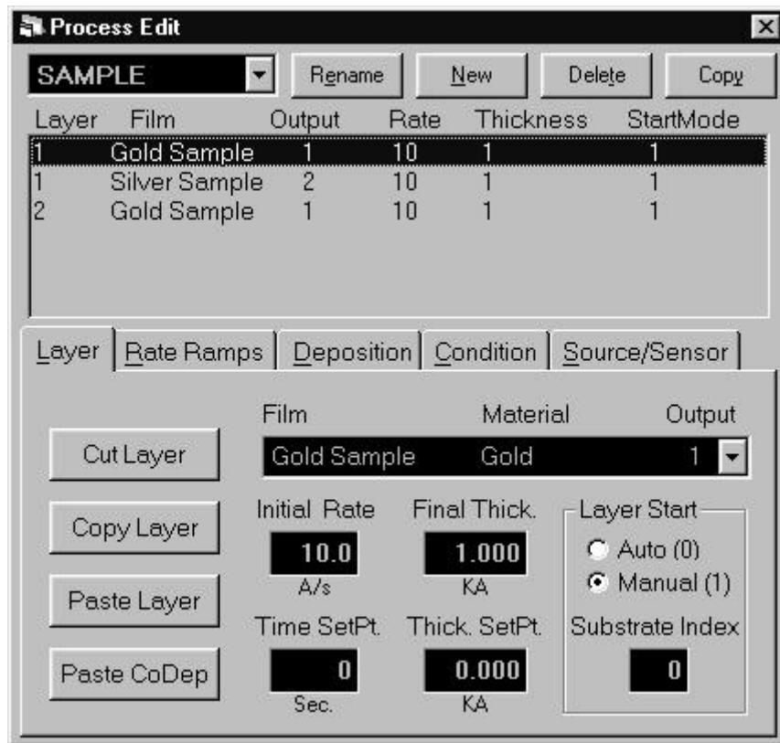
**Cut Layer:** Removes the layer selected in the Layers list box from the process, and places the layer on the clipboard.
