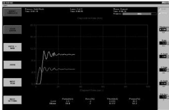
Included with the SID-142 is Sigma's SQS-142 software, a Windows-based program that provides all of the functions required for an eight sensor, four output, codeposition process. It is optimized for use with the Setting Knob and six SoftKeys of our SID-142 controller. However, it will run on any Win9X system with our SQM-142 card installed.
