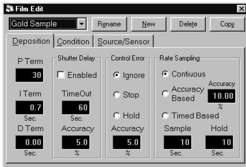
**Film:** A drop down box that selects the film parameters displayed in the edit film dialog box. Defaults to the current process film.
