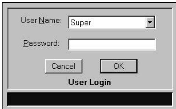
*Note: The SQS-142 software ships with one pre-assigned user. The user name is Super, with no Password.*
