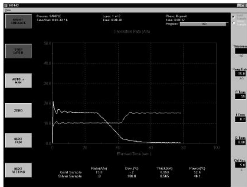
At .400kA thickness, the Silver Sample deposition rate ramps down from 15A/s to 0. Similarly, at .400 kA thickness the Gold Sample film ramps to a higher deposition rate of 15A/s. Because the initial rate for Gold was set lower than the initial rate for Silver, Gold reached its .400 kA thickness rate ramp trigger later in the deposition cycle.
