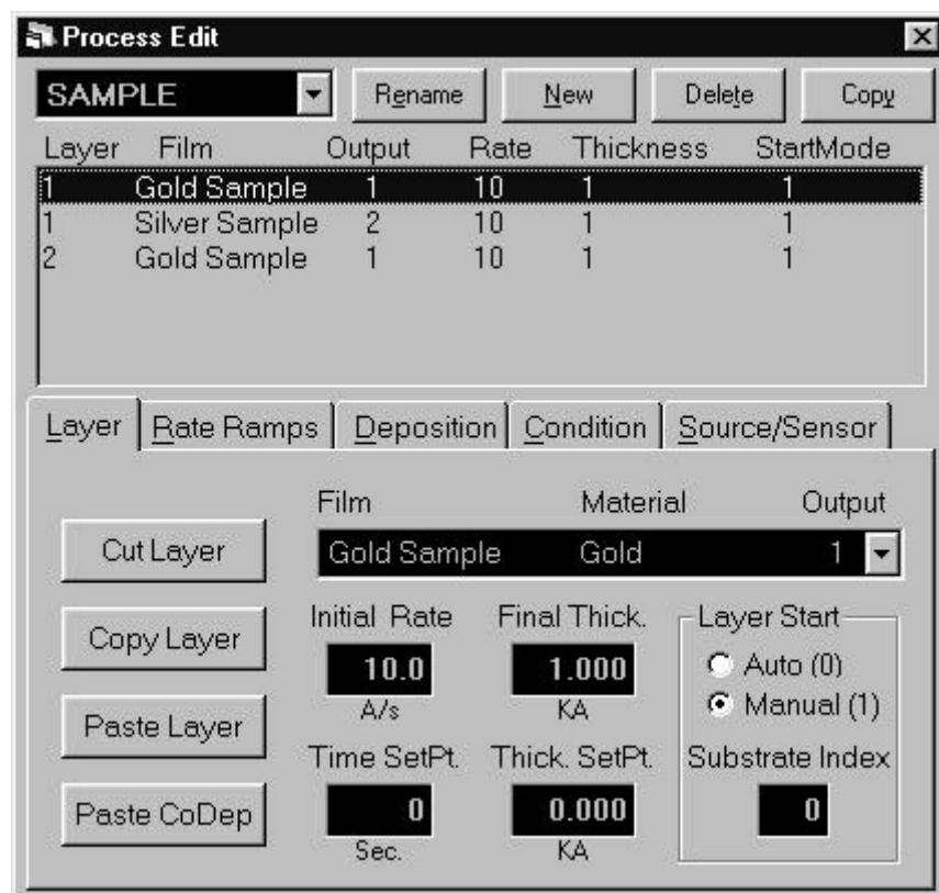
We now have two layers in our process. Layer 1 has Gold being deposited from source Output 1 and Silver is being codeposited on Output 2. Layer 2 is Gold alone.
