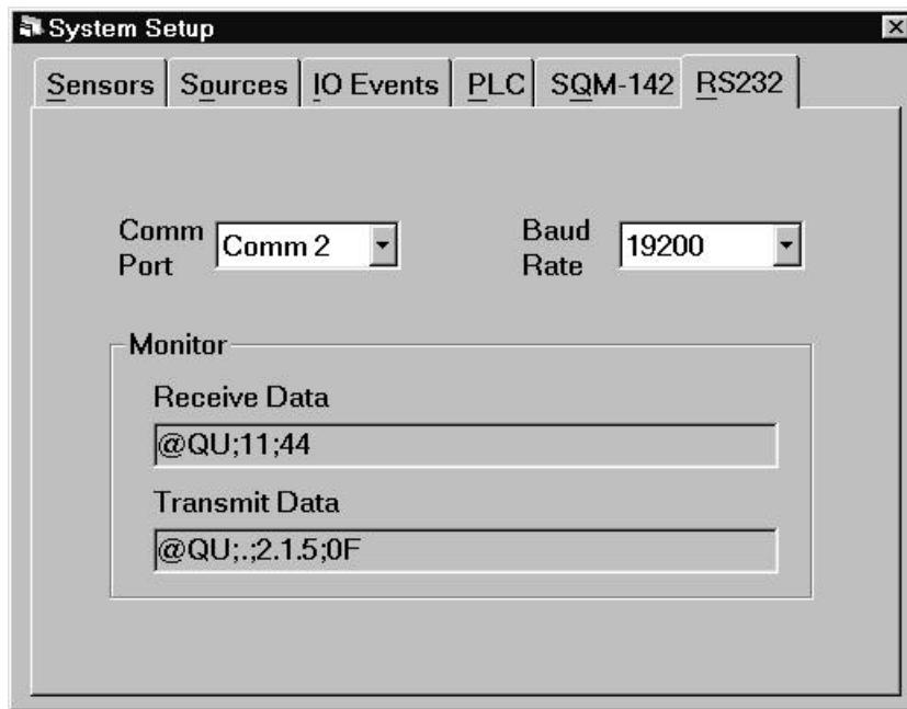
**Comm Port:** Selects the comm port used for serial communications. The Comm Port drop down lists available ports. However, some of the ports may be used by other devices (PLC, modem, mouse, etc.).
