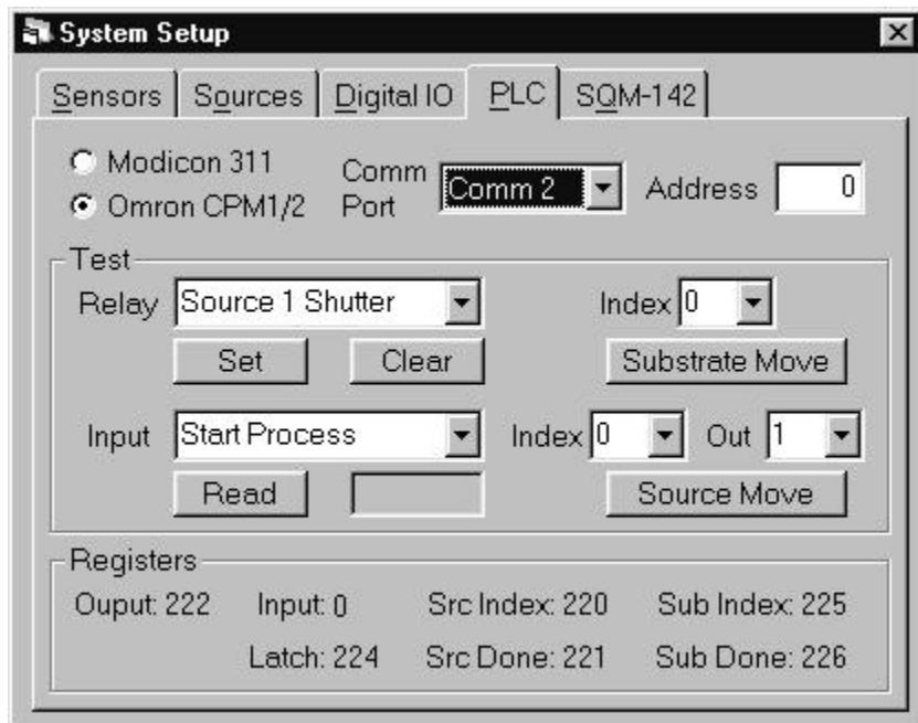
**Model:** Two models of PLC are supported. Select the model you are using.
