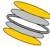
Full Pad Both Sides crystals have a fully-coated electrode on each side. These crystals do not require a specific orientation when installed. Full Pad Both Sides crystals are suitable for high volume production applications where maximum crystal life is not required. The Full Pad Both Sides design results in somewhat shorter crystal life and possible coupling of unwanted modes of oscillation. These unwanted modes can cause rate noise to appear earlier in crystal life.
