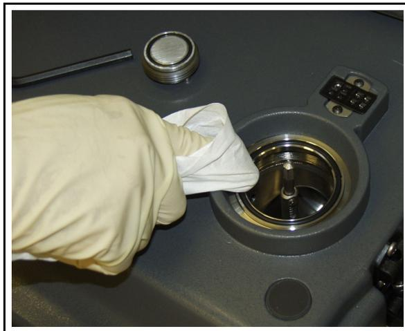
After cleaning, look for any visible cracking of the O-ring. If the O-ring is damaged, see [section 6.5.1, Replacing the O-ring, on page 6-5](#).
