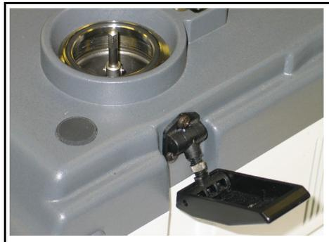
**NOTE:** Latches can be adjusted to the proper tension using the thumb screw.
