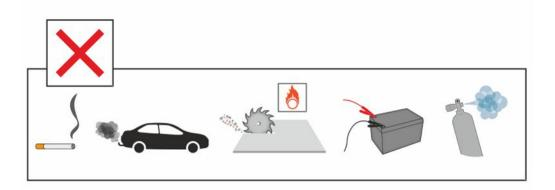
Avoid to place the instrument close to hydrogen sources such as cigarette smoke, combustion engines, aluminium machining, lead battery charging stations and, in some cases, compressed air systems.
