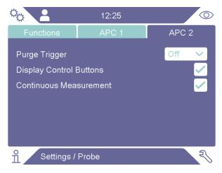
The Purge Trigger level can be set to the alarm level or a factor thereof. The factors that can be chosen are 1,5x, 2x, 5x, or 10x the alarm level.
