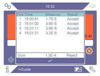
The summarized result will only be shown if the Reject on Sum function has been set. The order in the list can be changed, by pressing the headers in the list on the screen.
