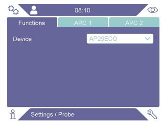
The task specific timers used in the AP29ECO sequence can be set in the "Settings > Probe > APC 1" menu. Further descriptions of the task specific timers can be found in the AP29ECO manual, see "Other associated Documents [▶ 7]".
