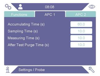
A Purge Trigger level can be set in the "Settings > Probe > APC 2" menu to protect the sensor from large tracer gas exposures.
