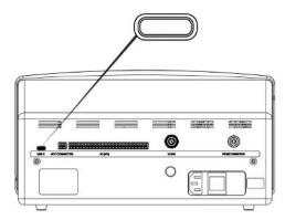
Connector:USB cablePurpose:For connecting the instrument to a PC or a USB-C mass storage device
