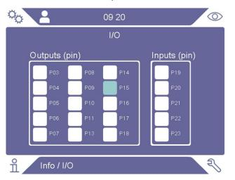
An output level high and output level low are marked with light blue and white color, respectively. See also the list of pins and functions in "I/O (APC) [> 66]".
