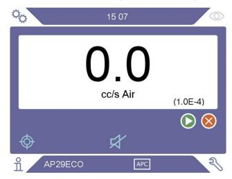
Activating the Continuous Measurement check box in the "Settings > Probe > APC 2" menu deactivates the Measuring Time parameter. The Measuring time is instead controlled by pressing the Start and Stop buttons on the Operations screen or by sending Start and Stop commands.
