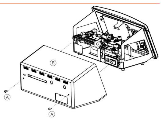
To change the battery remove the cover first.
