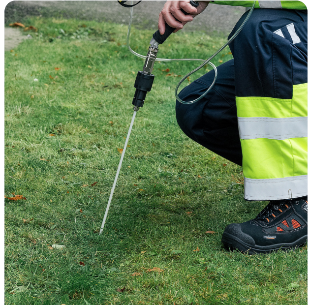
A pipe connected to a hose is a basic mean of picking up samples from the ground.
