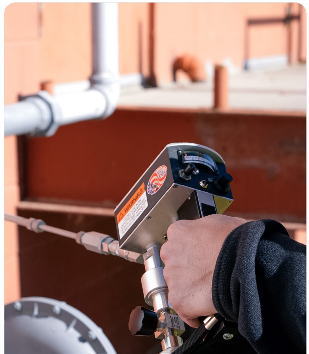
A flame ionization detector for finding natural gas leaks.
