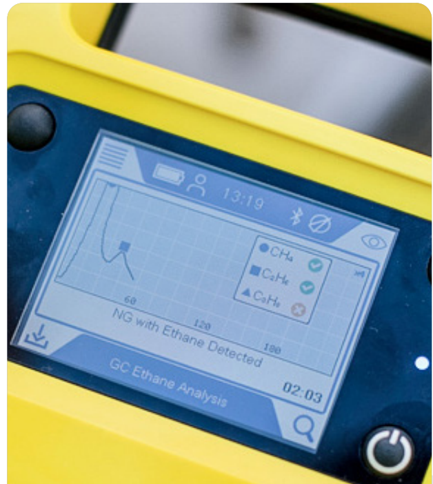
Built-in gas chromatograph allows for on-site gas analysis.
