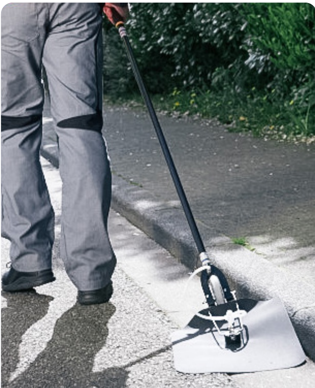
In a carpet probe, the end of the probe rests on a wheeled support, covered by a rubber mat.
