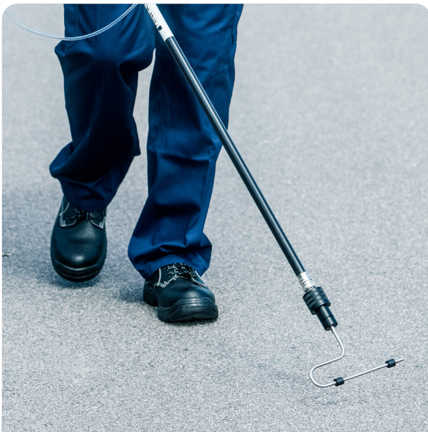
Inspection with an aerial-shaped ground probe can lead to inconsistent results due to difficulty in maintaining a consistent height.
