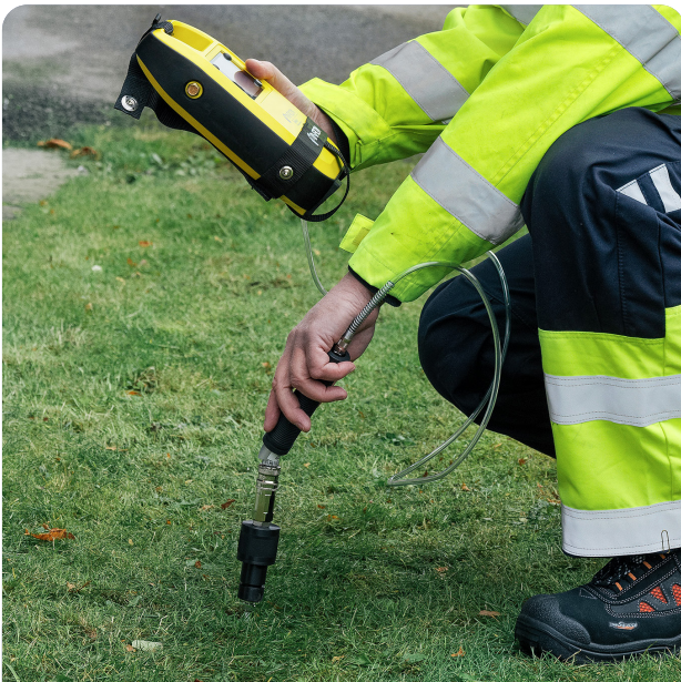
Inspection can be performed with help of bar holes in order to determine where the area of highest concentration is.
