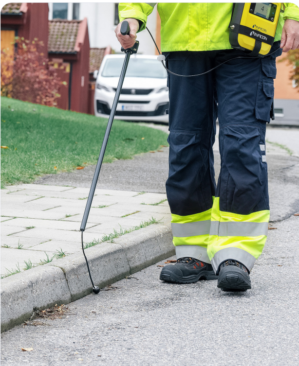
The use of the soft surface probe allows to collect a sample while walking.
