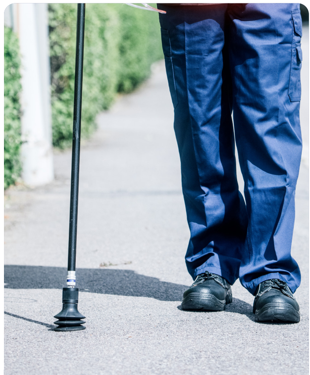
Inspection with a rubber bell, holding the probe like a ski pole and tapping the ground while walking forward in a Nordic style.
