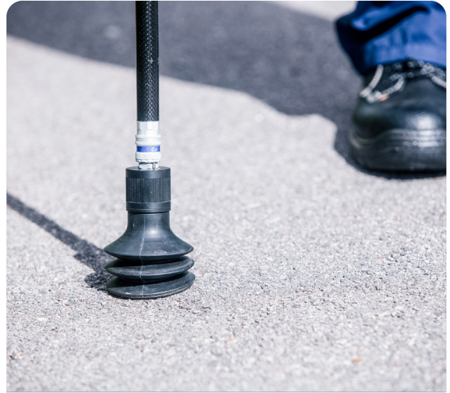
The vacuum bell forms an airtight seal against the ground and forces air to rise through the road surface.
