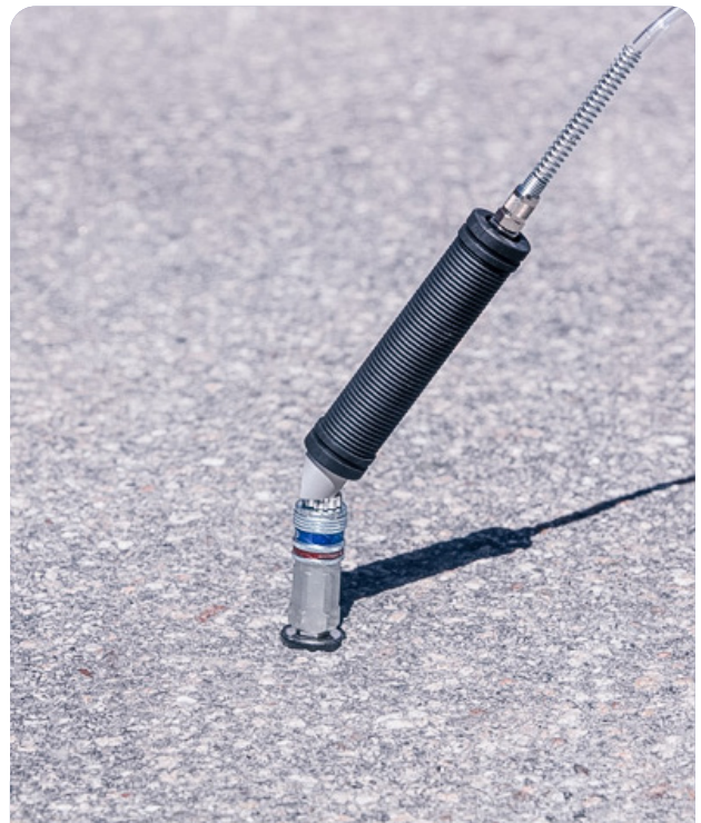
Gas samples are taken from the holes to identify the highest concentration location.
