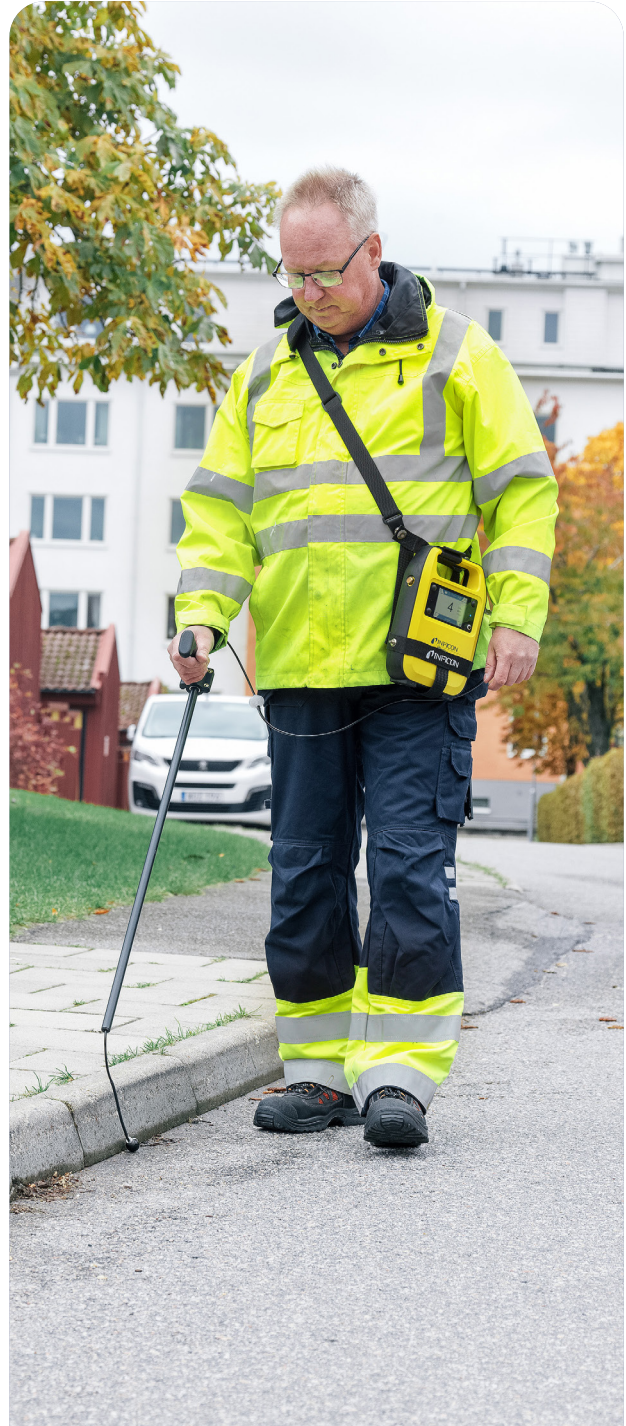
Successful gas detection also depends on the method by which the gas is picked up from the ground.
