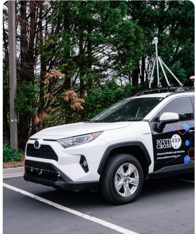
A vehicle-based leak survey system using sensors and equipment mounted on a vehicle to detect gas leaks.
