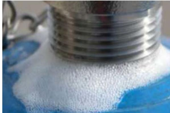
A simple procedure: soap testing of a threaded connection
