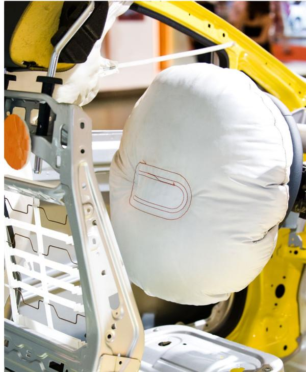
Using the bombing method, airbag igniters are tested against a leak rate of  $10^{-6}$  mbar·l/s
