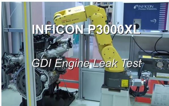
[Robotic leak testing on GDI engines](#)
