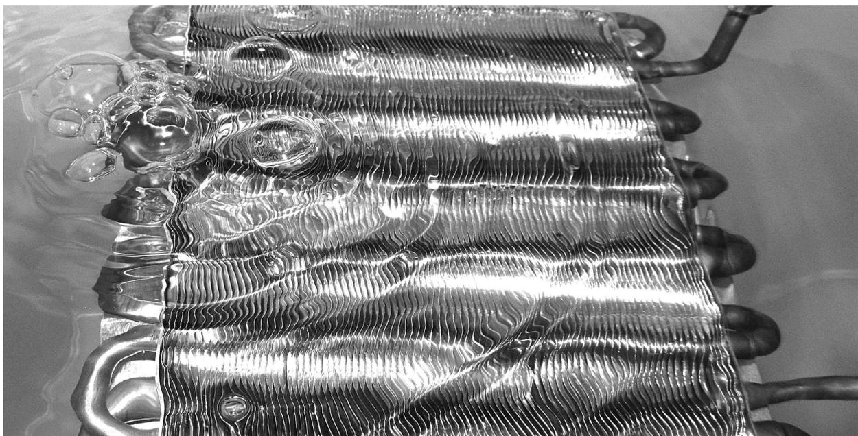
The detection limit of bubble testing deteriorates depending on the geometry of the test piece
