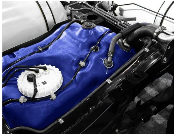
For testing a truck's fuel tank against leak rates up to  $10^{-4}$  to  $10^{-6}$  mbar·l/s neither bubble tests nor pressure decay tests are sensitive enough
