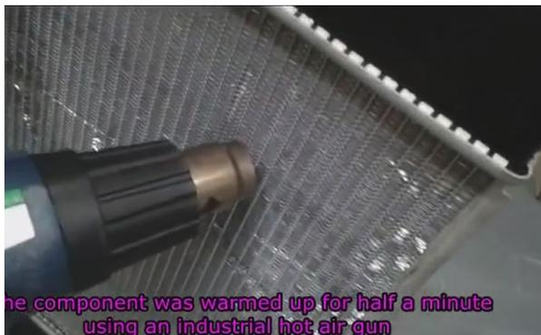
[Leak testing of evaporators for car A/C with T-Guard](#)
