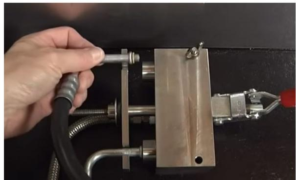
[Leak testing of car A/C hoses](#)
