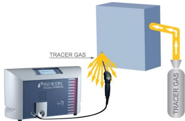
Sniffer leak testing (with manual sniffer probe) finds the exact location of a leak
