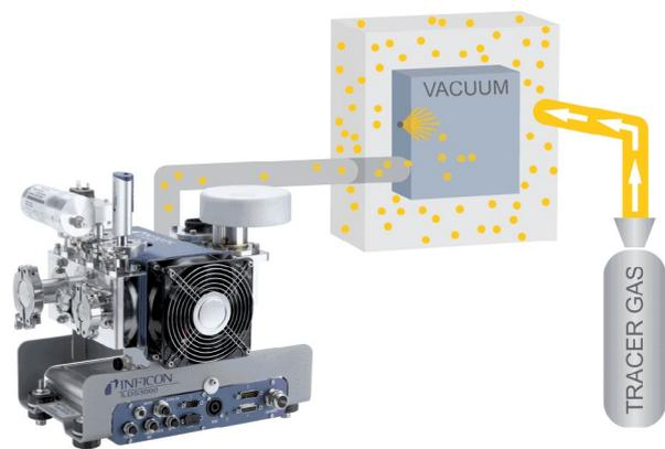
Vacuum leak testing (with vacuum in the test piece) is often well suited for production line testing
