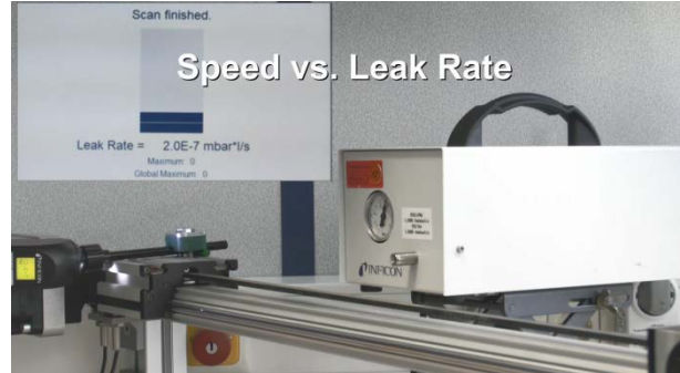
Setup for dynamic testing: sniffer tip is moved across a test leak opening with constant transversal speed (Click on picture to see video illustrating the testing cycle on YouTube)
