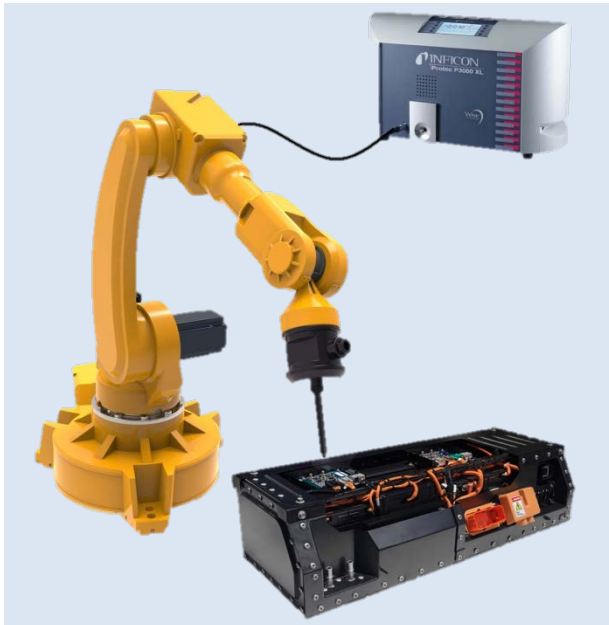
Example of a robotic leak testing application: A robot is sniffing potential leak locations on a battery pack housing
