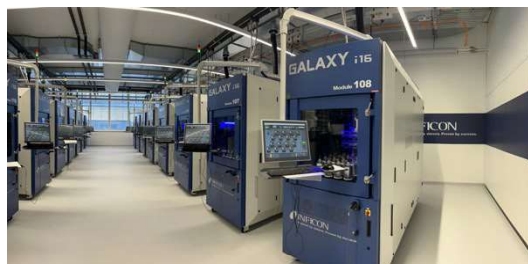
Vacuum gauge calibration systems, Balzers (LI)
