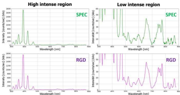
The optimized gas spectrum allows the precise testing of existing gases in the vacuum system and the measurement of gas partial pressures. This is how the OPG550 sensor allows
