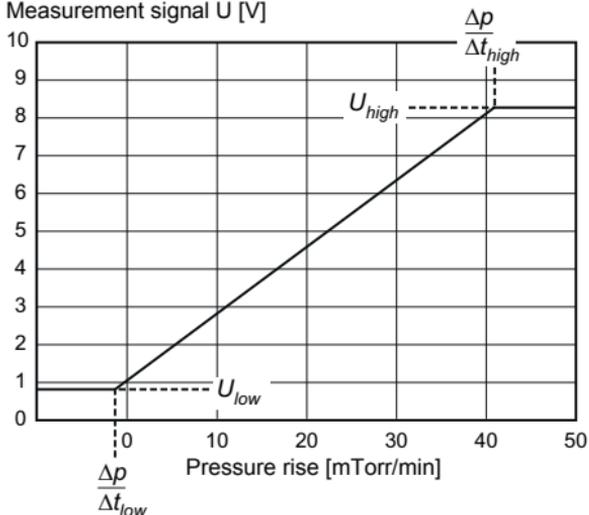
$$U[V] = m \frac{\Delta p}{\Delta t[mTorr/min]} + n \quad \Leftrightarrow \quad \frac{\Delta p}{\Delta t}[mTorr/min] = \frac{U[V] - n}{m}$$
