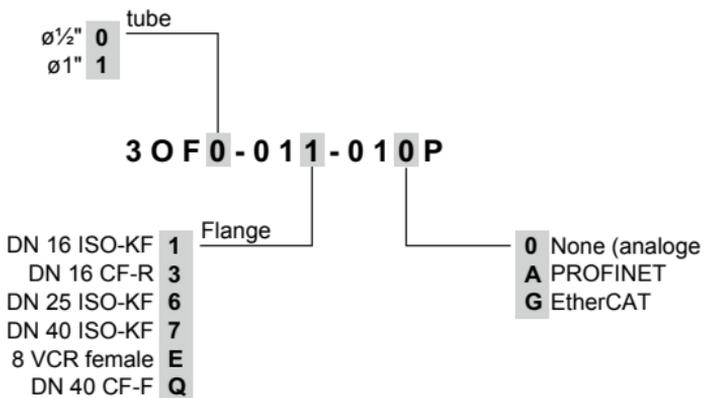
The part number (PN) can be taken from the product nameplate. If not indicated otherwise in the legends, the illustrations in this document correspond to gauges with DN 25 ISO-KF vacuum connection. They apply to gauges with other vacuum connections by analogy.
