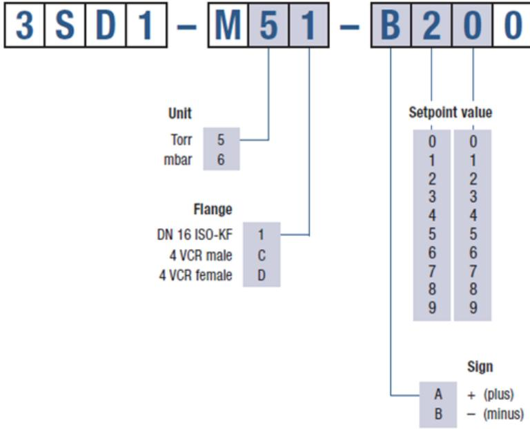
Example: 20 Torr below ambient pressure, DN 16 ISO-KF: 3SD1-M51-B200
