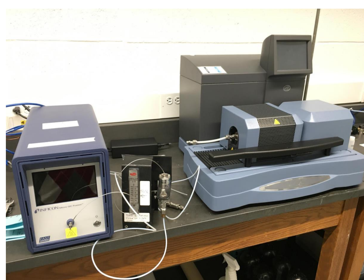
Figure 4: TGA/DSC connected to the Micro GC gas analyzer
