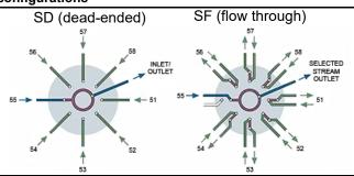
INFICON offers a 10-port SD (dead-ended) and a 10-port SF (flow-through) Valco stream selector accessory package pre-assembled from the factory. The pre-assembled Valco stream selectors have 1/16 in. sample line filters installed and leak checked at each inlet port. (See Figure 3.) Simply connect the sample lines and the Valco stream selector is ready to use.
