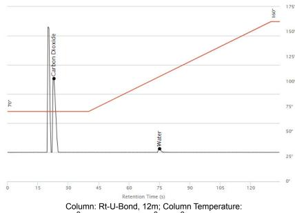
Figure 4 Chromatogram of Module B with Water in Sample (Helium)
