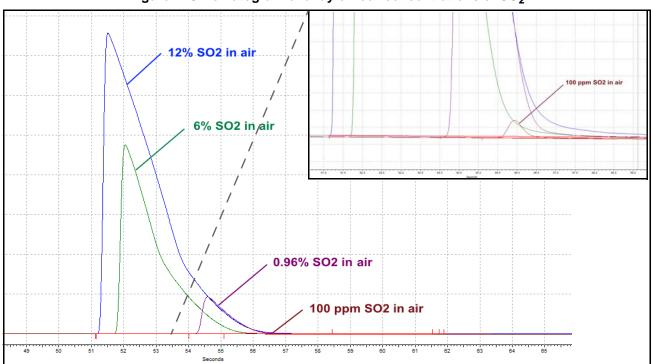
Figure 2 Chromatogram overlay of four concentrations of SO<sub>2</sub>
