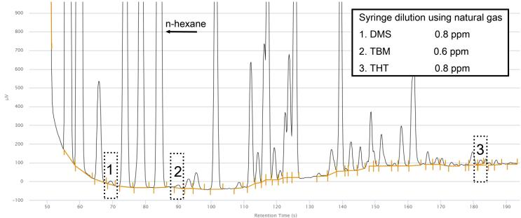
Micro GC Fusion was connected to a natural gas pipeline source to measure odorants in a natural gas stream. The results show 1.2 ppm of DMS and 2.0 of TBM. THT was not present in the sample.
