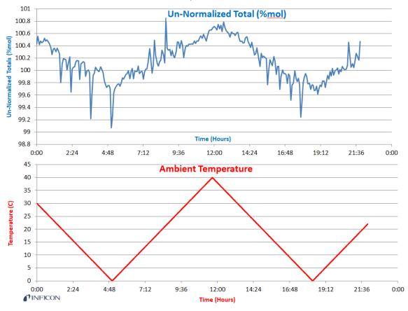
Area counts remained stable over the course of the experiment and met the <1% RSD specification for area stability.
