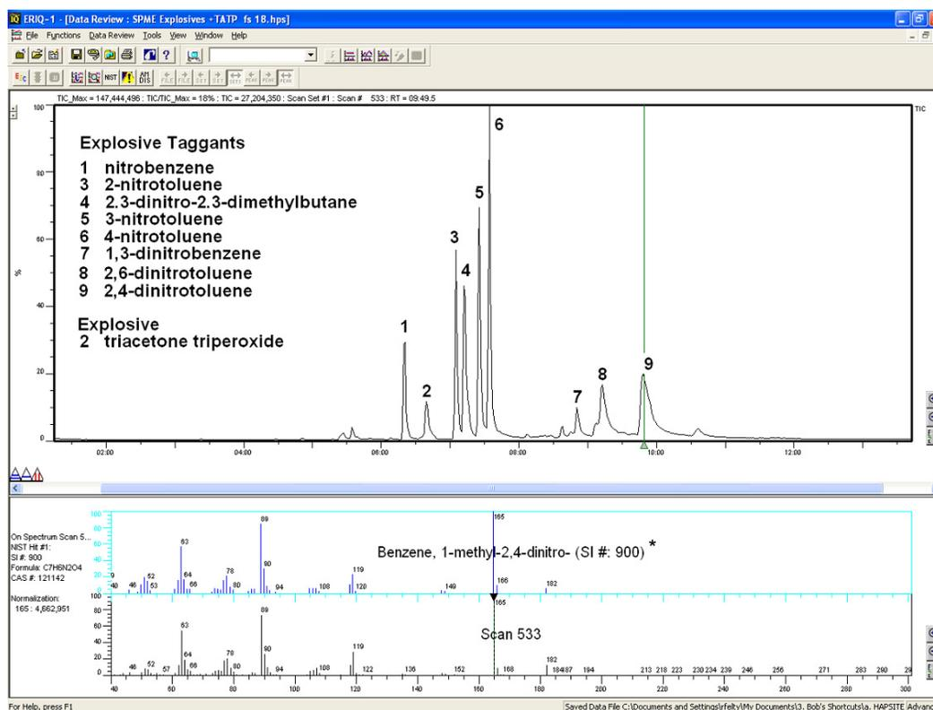
Column: Rtx-1MS (15 m x .25 mm x 1.0  $\mu$ m)
