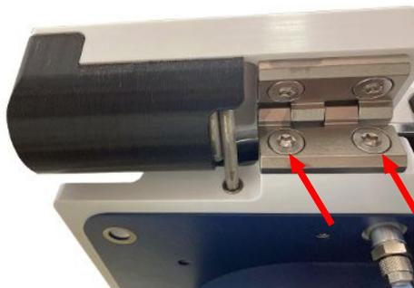
Fig. 14: Fastening to lower membrane support
