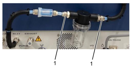
Fig. 11: Change liquid separator
