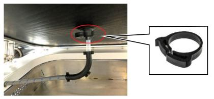
Fig. 8: Ratchet clamp on the underside of the measuring chamber
