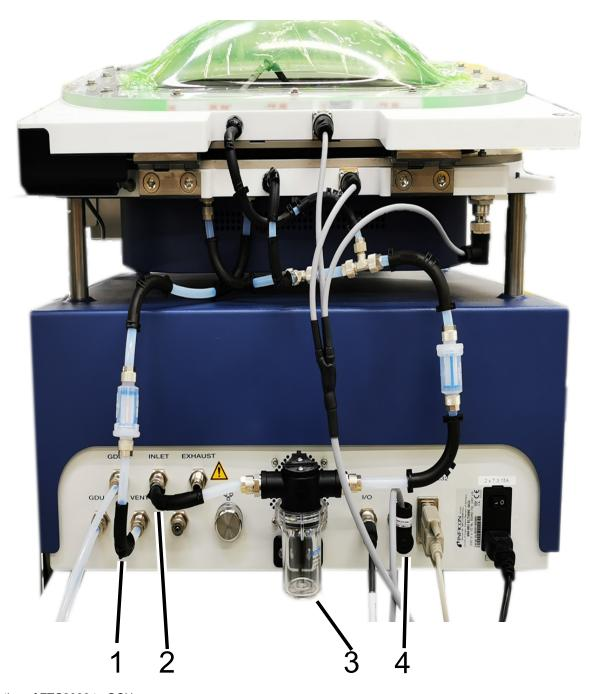
Fig. 3: Connection of FTC3000 to GCU
