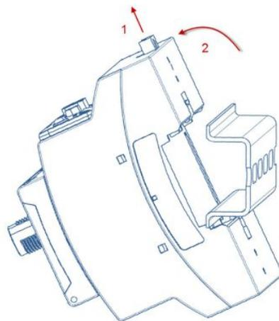
Fig. 3: Remove IC1000
