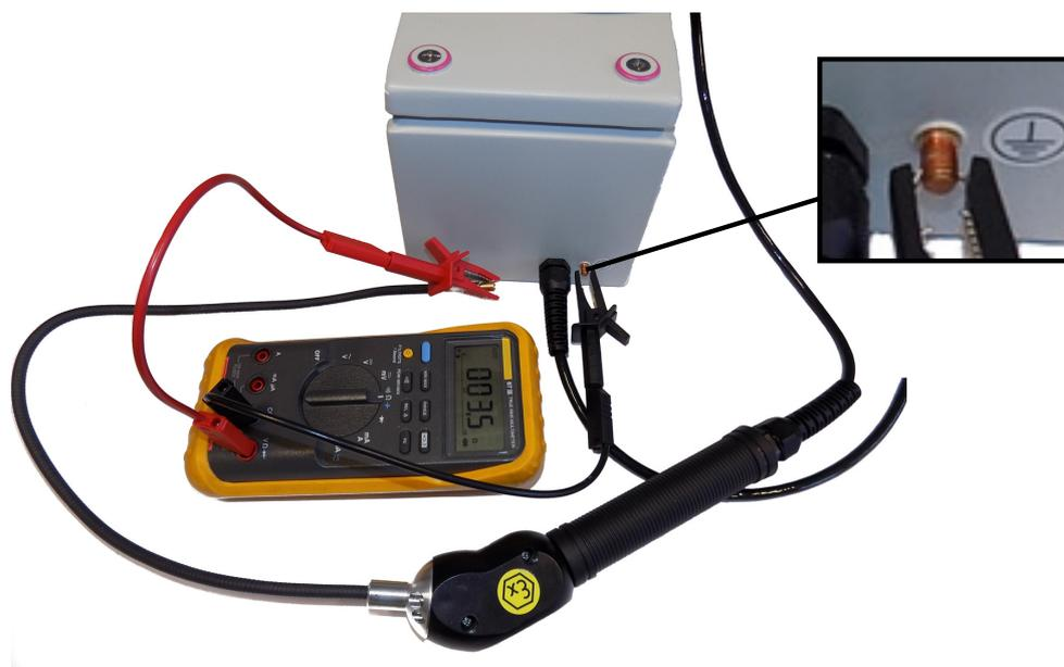
Fig. 3: Checking connection between capillary filter and ground
