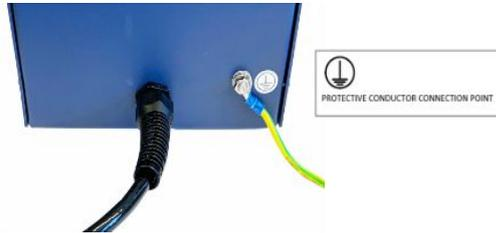
Fig. 1: The grounding cable (here yellow-green) must be attached to the protective conductor connection of the interface box using the preassembled washer and nut!
