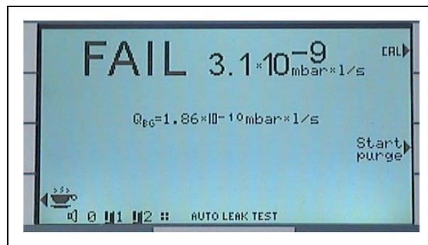
Fig. 3-7 Trigger level set to  $1 \times 10^{-9}$ , a leak found
