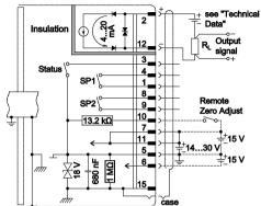
If no sensor cable is available, make one according to the following diagram (cable length and conductor cross-sections  $\rightarrow B$  11).
