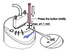
... apply supply voltage to Remote Zero at pin 10 (pulse  $\rightarrow \mathbb{B}$  10).
