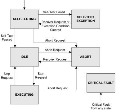
**Abort** - Used to transition the device application objects to the aborted state. This service request may be (and generally will) originated internally, from application objects.
