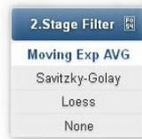
In situation of very long static measurements, the data can be further smoothed by applying a secondary stage filter. If a Second Stage Filter is applied, the CDC and the Adaptive Filter settings are adapted accordingly.
