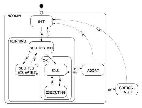
After the start, the gauge independently runs through the INIT and SELFTESTING status and eventually changes to the IDLE status (if there is no error) or to the SELFTEST\_EXCEPTION status (if there is a gauge error).
